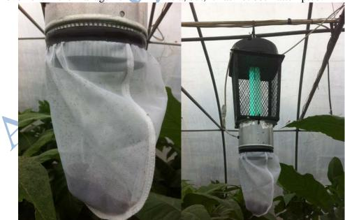
The trap is a modified "bug zapper" with the bottom removed. A downward throwing "duct booster" fan is duct tapped to the bottom and the power for the fan is take
