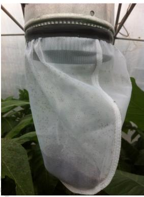
The trap is simply a modified "bug zapper". We remove the bottom plate and duct tape a "duct booster fan", blowing down, to the bottom of it. The wiring in the bottom of the "zapper" is tapped into for the "duct fan". We then use an elastic band to hold a "paint straining bag" onto the discharge end.
